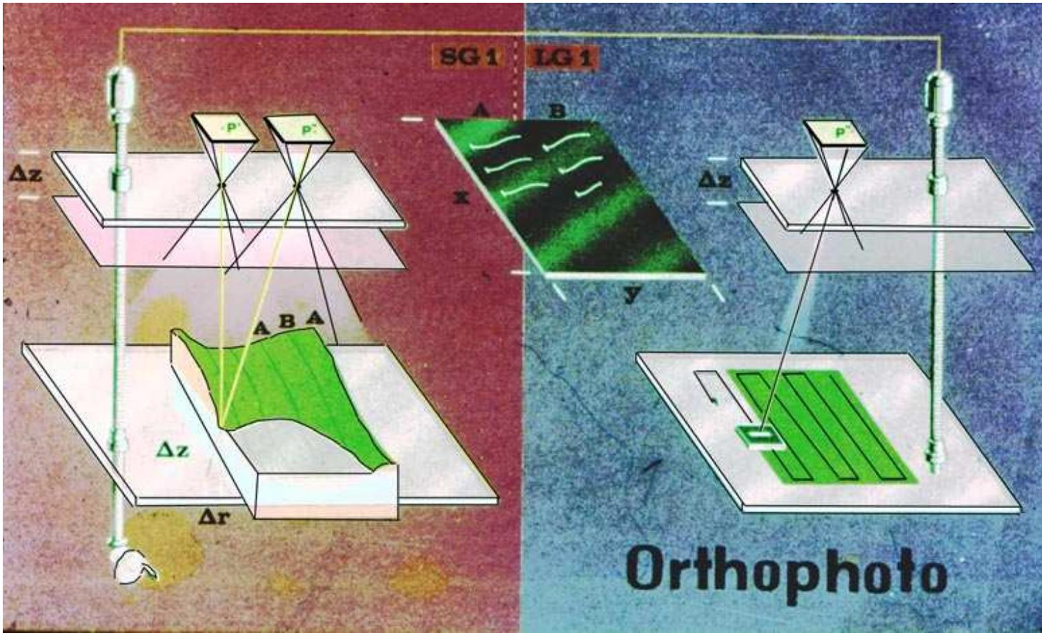
Differential transformation (processing) – using analog instruments
